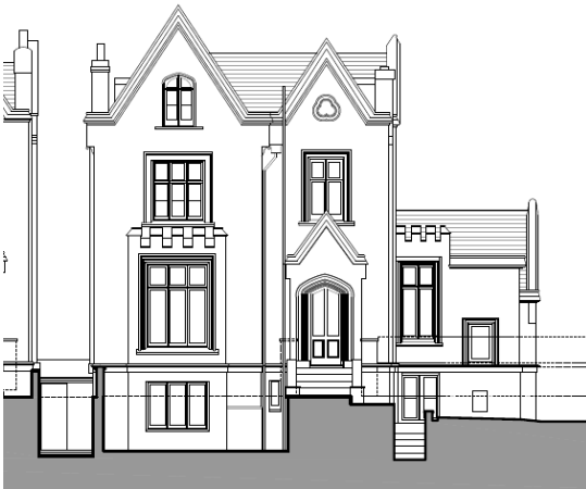
Existing South East Elevation - Clifton Hill 1:100
